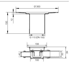
Floor drain set DN 50/70 with odour trap, Drain DN 50 (50 mm) with rigid connector, Drain capacity according to DIN EN 1253: With 2 cm head of water = 0.8 l/s (48 l/min) With 1 cm head of water = 0.65 l/s (39 l/min) Water trap height: 5 cm Art. No. KD BH 5070 GVB Supplied unit:
