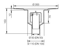
Thin-set floor drain set DN 50 with odour trap Drain DN 50 (50 mm), Drain capacity according to DIN EN 1253: With 2 cm head of water = 0.6 l/s (36 l/min) With 1 cm head of water = 0.55 l/s (33 l/min) Water trap height: 3 cm Art. No. KD BV 50 GVB Supplied unit:
