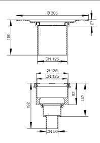
Floor drain set DN 50 without odour trap with sealing flange
