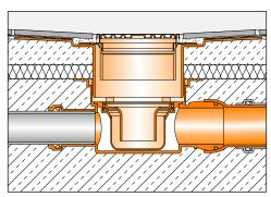
Fig.: Frame with conventional grate cover and odour trap unit
