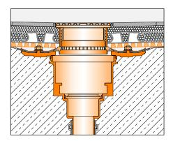
Application: Exterior (2-level drainage, loose installation)
