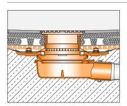
Application: Exterior (2-level drainage, loose installation)
