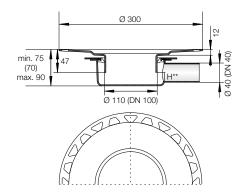
Floor drain set DN 50 with odour trap Inlet DN 40 (40 mm), outlet DN 50 (50 mm) with pivot connection Drain capacity according to DIN EN 1253: With 2 cm head of water = 0.6 l/s (36 l/min) With 1 cm head of water = 0.55 l/s (33 l/min)
