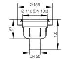
Thin-set floor drain set DN 50 with odour trap Drain DN 50 (50 mm),
