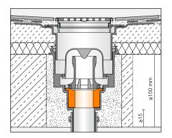
Fire protection insert KERDI-DRAIN-BS
