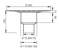
Floor drain set without odour trap Drain DN 50 (50 mm), Drain capacity: 1.4 l/s (84 l/min) with grate/frame combination Grate D
