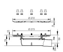
Floor drain set DN 50 without odour trap with sealing flange to create 2-level drainage of surface water and seepage
