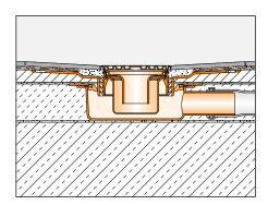
The installation height can be reduced by 5 mm to 70 mm by removing the rubber ring. To meet the requirements of DIN EN 1253 and to achieve a drain capacity of 0.4l/s, a free cross-section (H\*\*) of 32 mm must be ensured. The thin-set insert and neck must be cut to size accordingly if a covering support is used.
